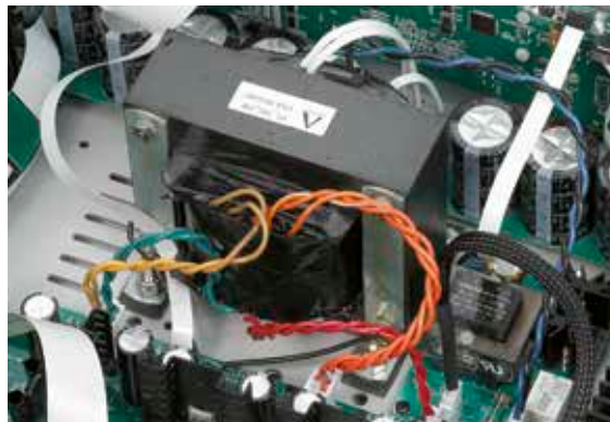
◀ Instead of the conventional, externally made toroidal transformer, Aesthetix uses a homemade one.
